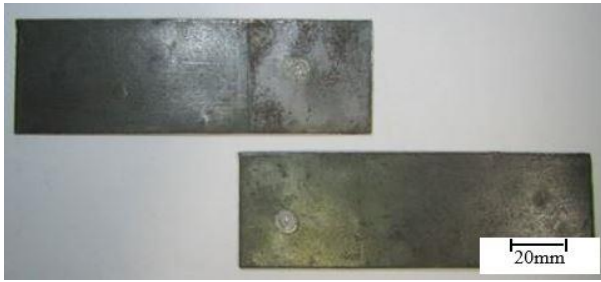
Fig.3(a): Joint failure mode: interfacial
