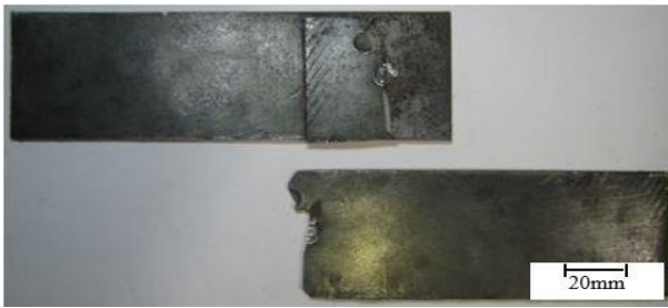
Fig.3(b): Plug failure mode
